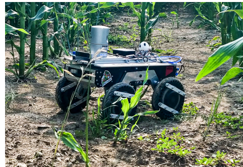
Fig. 1. Image of the developed robot navigating a crop field.
