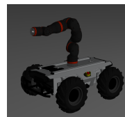
Fig. 1. Igus Rebel and Agilex Scout in Gazebo simulator
